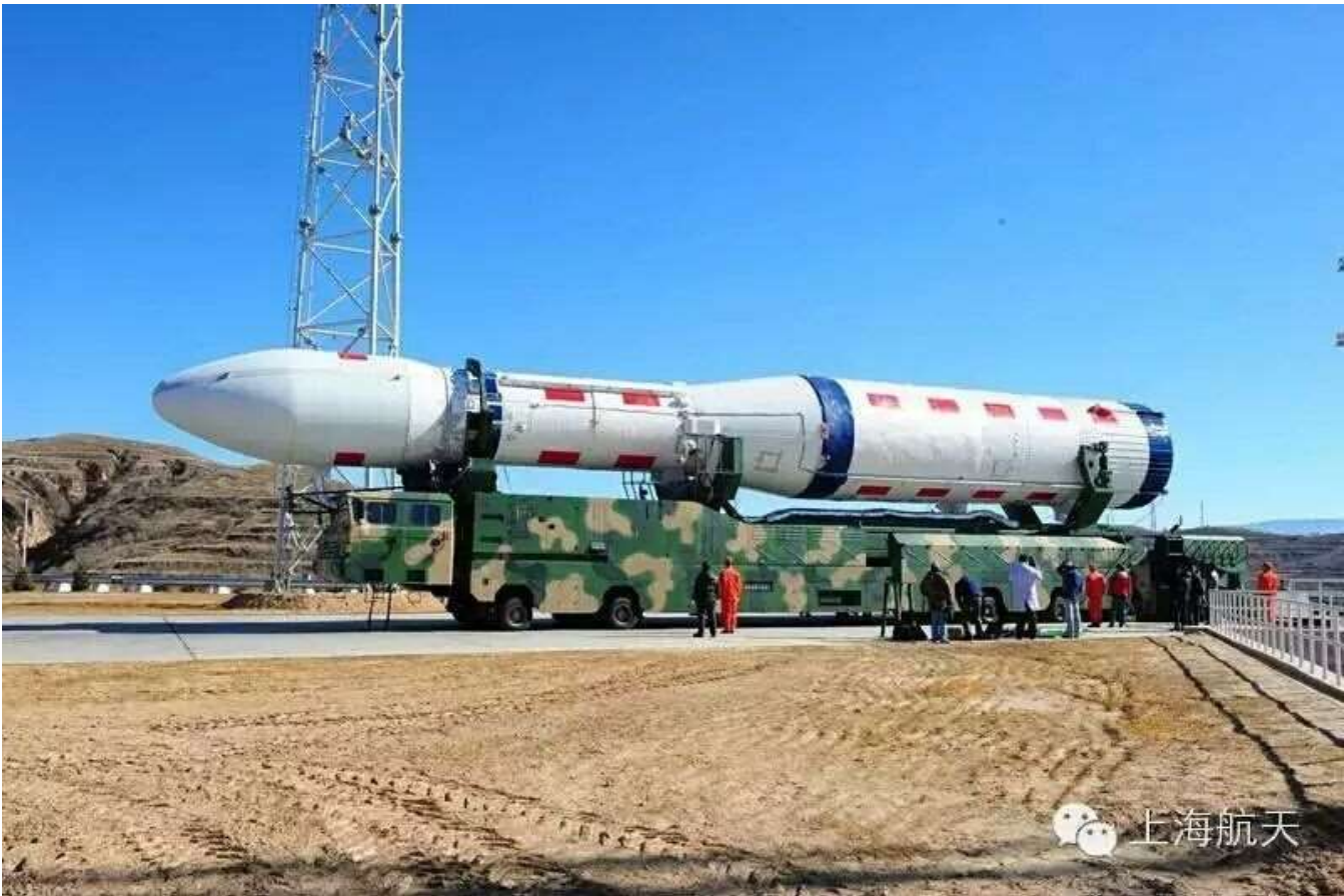
Fig. 3 , the CZ-6 rocket on a camouflaged TEL. (Photo credit: watermarked WeChat user)
